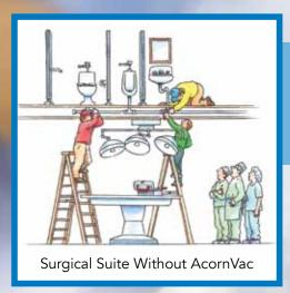
**GRAVITY PLUMBING** requires that contractors have access to the space below the floor.
