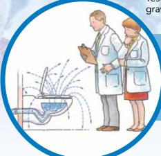
**GRAVITY TOILETS** produced **detectable levels of overspray and bacteria** on the toilet seat and in the area surrounding the toilets.
