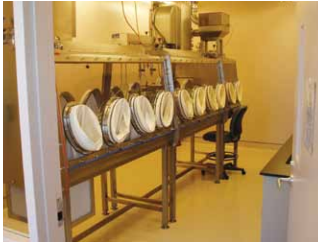
Left: In the BSL-3 lab, researchers conduct experiments on contagious materials in gas-tight enclosures, thus the need for a fail-proof wastewater system. Right: The two 60-gallon vacuum system tanks collect wastewater 8 feet above the ground.
