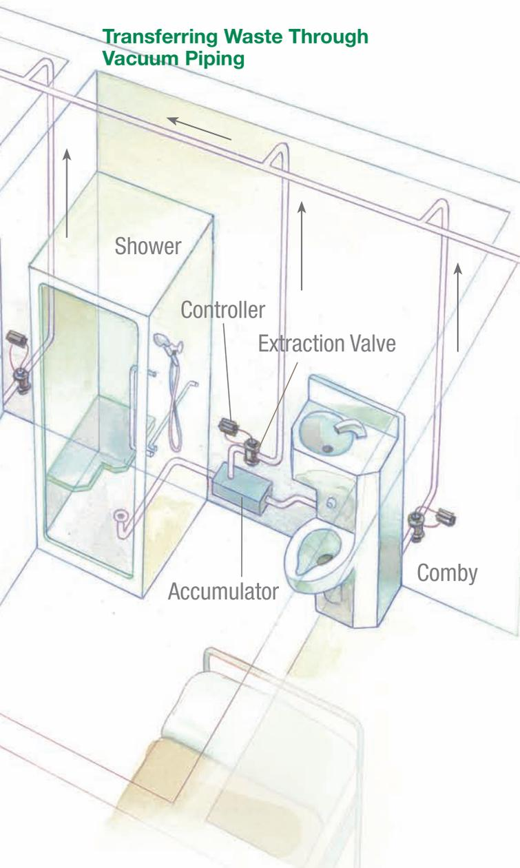
**Transferring Waste Through Vacuum Piping**
