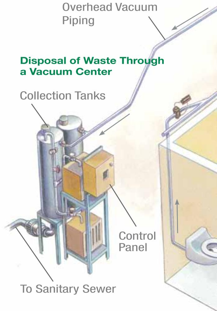
**Collection of Wastewater Through Fixtures and Accumulators**
